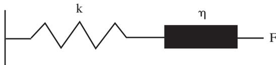
In this model, the stress provided by each force is the same, and the elongation of the material under constant stress is:
